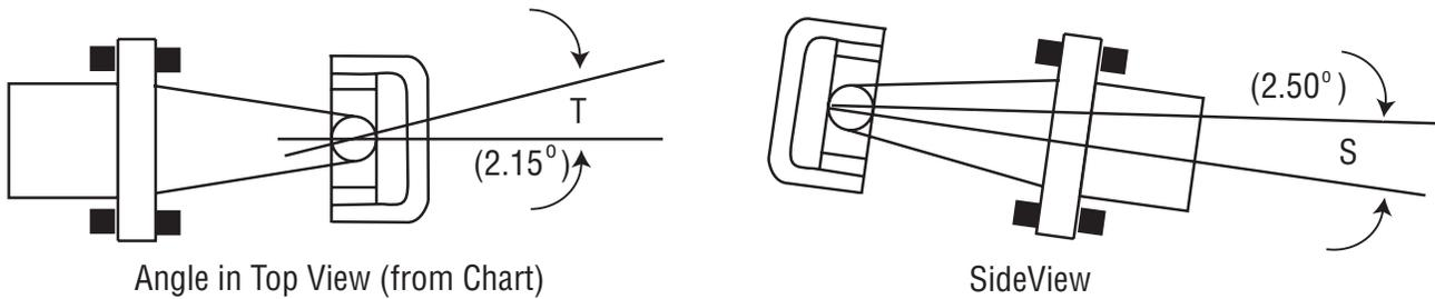
$$\text{Compound Angle } (C^\circ) = \sqrt{T^2 + S^2}$$
